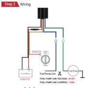
NOTE A A : After installed SIM card correctly , it is very important to connect the tracker with external power no less than 12V for power supply before operation!
