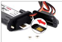
2. Plug-in SIM card (SIM card not include)
