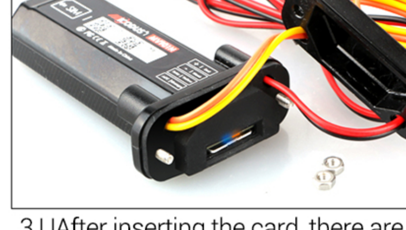
3.UAfter inserting the card, there are blue and orange LED lights flashing respectively.
