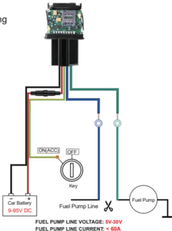
**NOTE** ⚠️⚠️⚠️ : After installed SIM card correctly , it is very important to connect the tracker with external power no less than 12V for power supply before operation!
